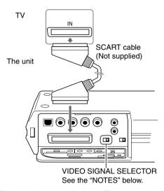
This illustration is upside down. (The bottom side is up.) For details on the connectors' name, see page 38.
